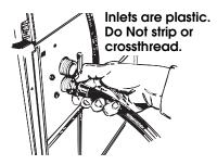
Attach hose to bottom inlet valve opening first. Then second hose to top inlet. Tighten couplings by hand; then use pliers to make an additional two-thirds turn.
